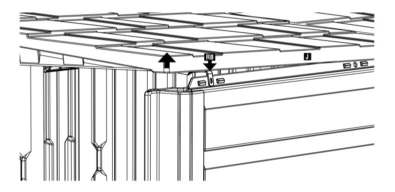
Make sure Front Roof (J) is positioned tightly against the middle Repeat Roof (M) section.
